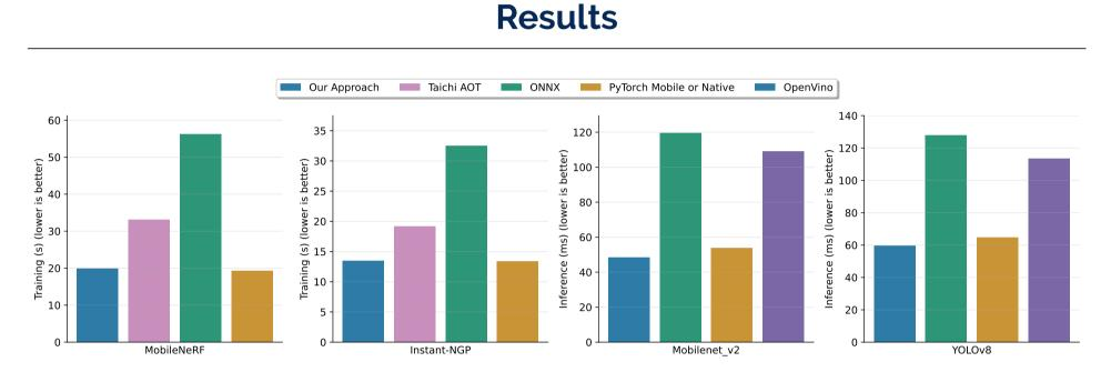
Figure 3. A quantitative comparison of how our approach relates to other edge deployment platforms, we use similarly quantized models to ensure fair comparisons. For MobileNeRF and Instant-NGP we compare our approach to Taichi AOT, ONNX, and a Native runtime. For MobileNet and Yolov8 models we compare our approach to OpenVino, ONNX, and PyTorch Mobile.
