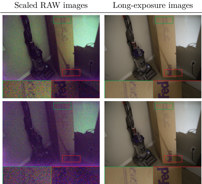
Figure 4. The scaled images and long-exposure ground-truth images for the same scene across three different low-light factors \times 100 (first row), \times 250 (second row), and \times 300 (third row) captured on Sony \alpha 7SII with an ISO of 10000.
